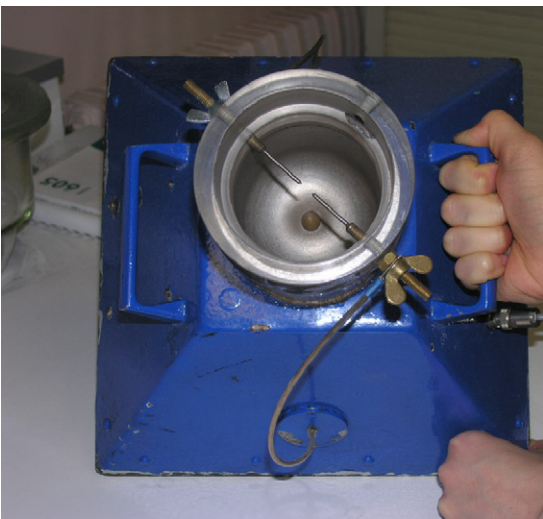
Fig. 1. View of the low bottom part of the HARTMANN apparatus (electrodes and dispersion mushroom) on the top of which the Plexiglas tube is settled prior to a test.
