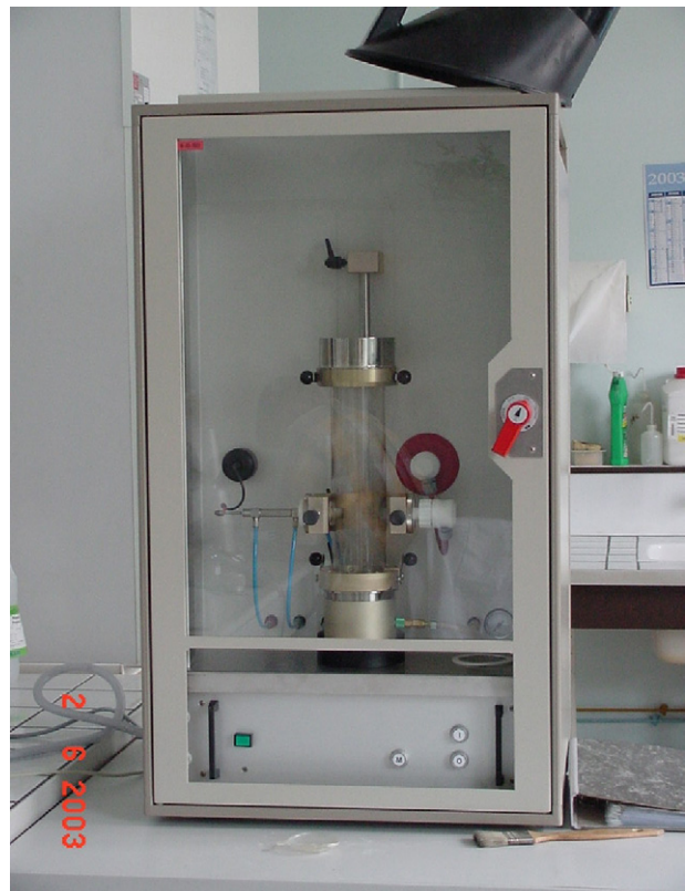
Fig. 3. Front view of the MIKE 3 apparatus.
